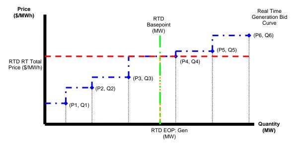
In the diagram below, however, the RTD interval LBMP intersects the given Generation Bid block on a horizontal line; however, the Generator was Base Pointed beyond its economics. In this case, the Generator's EOP is equal to the higher Generation Block MW (i.e.,  $Q_4$ ) of the block where the RTD interval LBMP intersects the Generation Bid.
