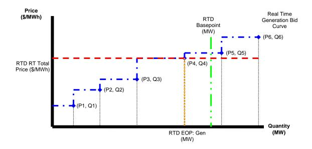
In the diagram below, the RTD interval LBMP intersects the given Generation Bid block on a horizontal line and the Generator was Base Pointed below the given Generation Bid block. In this case, the Generator's EOP is equal to the lower Generation Block MW (i.e.,  $Q_3$ ) of the block where the RTD interval LBMP intersects the Generation Bid.
