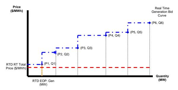
If the RTD interval LBMP (i.e., RTD RT Total Price (\$/MWh)) is greater than the cost component of the last point on a Generator's Bid curve, depicted as P<sub>6</sub> in the diagram below, then the Generator's EOP is equal to the megawatt component of the last point on the its cost curve (i.e.  $Q_6$ ).
