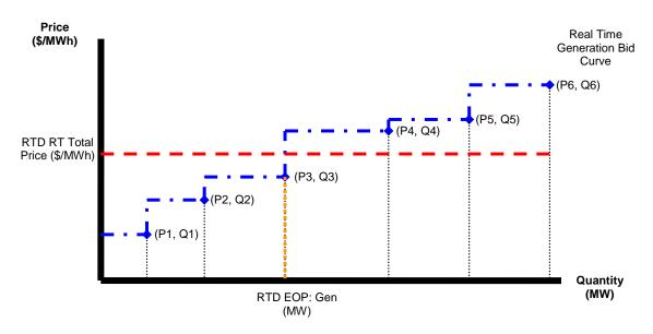
If the RTD interval LBMP intersects the given Generation Bid block on a horizontal line and the Generator's RTD Base Point is greater than the megawatt component of the last point on the Generator's Bid curve, as in the diagram below, then the Generator's EOP is equal the its RTD Base Point.
